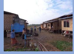
A new community built in just 3 months : The people staked out the plots, constructred the infrastructure (with water pumps, toilets, shared septic tanks and simple raised earth lanes) and built the houses themselves, in sub-groups, very simply and well. They figure that these simple houses will last about 7 years, when they'll be better-off and be able to upgrade them.
