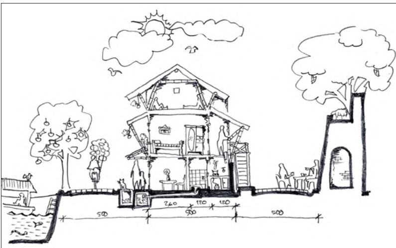
▲ This drawing depicts the concept of the prototype housing design, which is situated between the river and the Old Wall. A wide promenade provides access to the water while also housing a utilities channel for drainage and septic tanks. Residents can enjoy a tranquil and shaded gathering space on the Wall side.
