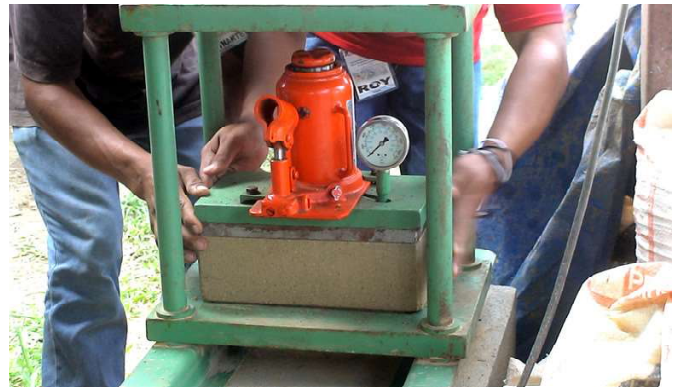
The finished blocks were periodically tested for compressive strength, which was almost always much greater than conventional concrete block.
