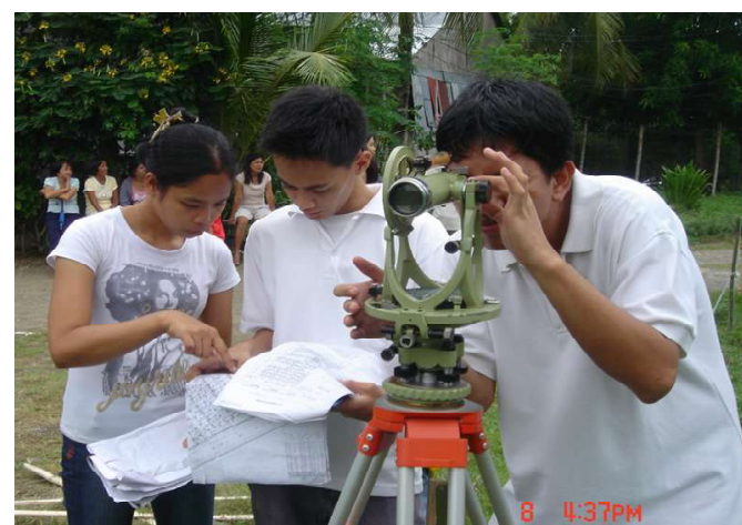
Once the subdivision plan was approved by the city, the architects and engineers surveyed the site, to mark out the house plots and roads, with assistance from students from nearby technical colleges
