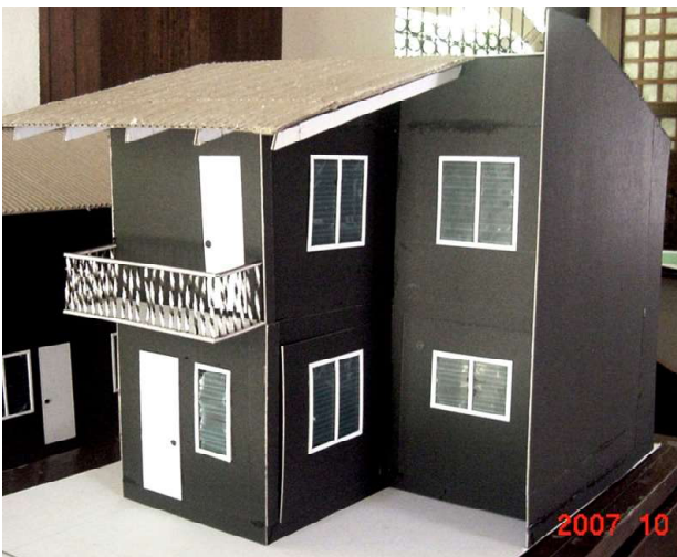
Here are models of two types of the detached single houses, which could be built within the CLIFF loan limits, if the lower floors were left unfinished. All the detached houses were designed to be built right on the property line, with fire walls, to save space for future additions.
