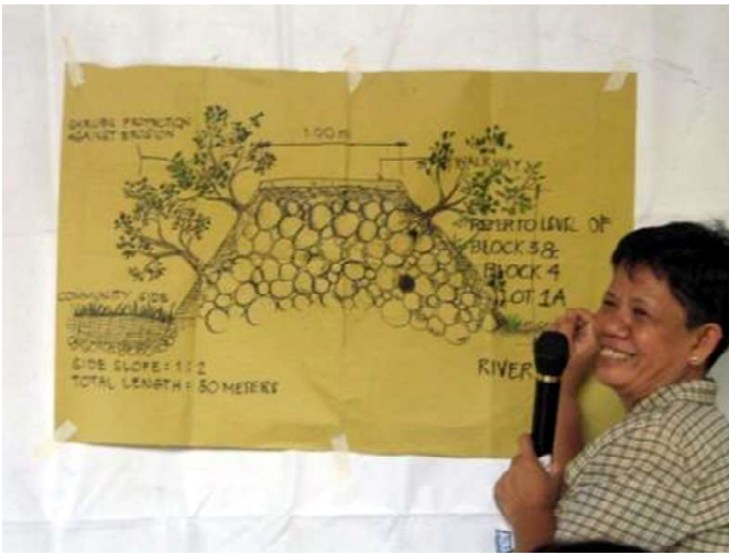
While the new houses were being built, the community decided to collectively design and build a 70-meter long earthen dike along the river side of the community, to protect it from flooding. Photos from the special earthen dike design workshop (left) and with architect May Domingo-Price on the site (right).
