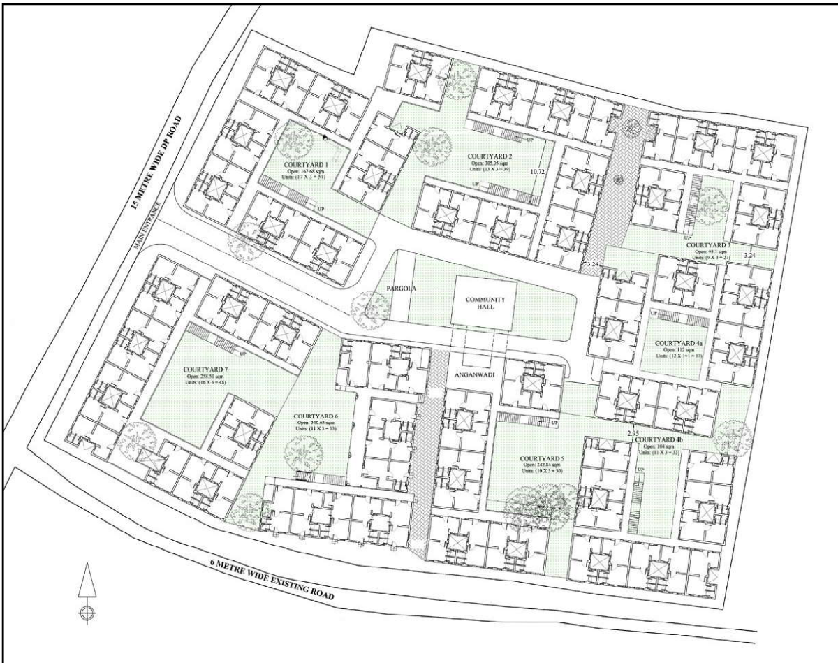
▲ Here is the final layout plan for the redevelopment of Sanjaygar, with each of the eight buildings arranged around its own courtyard - carefully designed to preserve all the mature trees.
