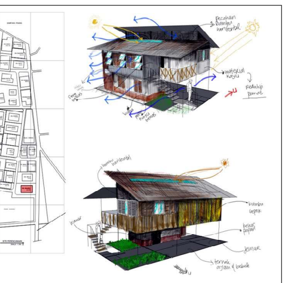
The community architects worked with every family to plan their airy, comfortable new houses, using as many materials salvaged from their old houses as possible, to save money.
