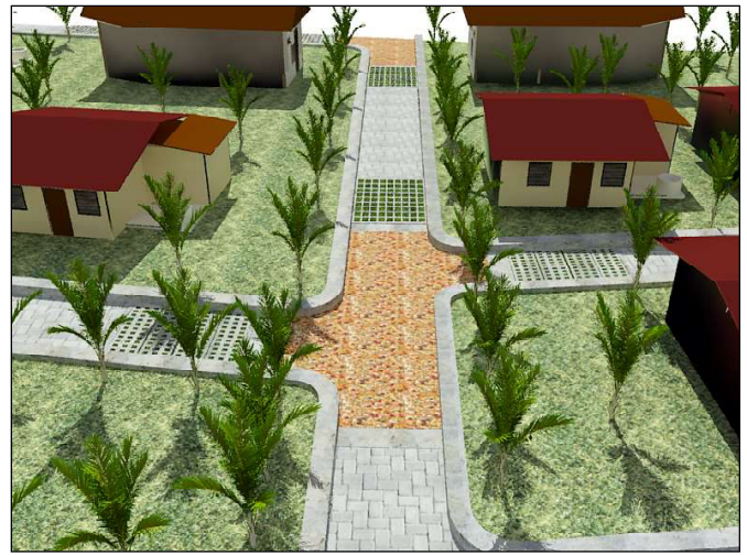
Besides the layout and the houses, the people also worked with the architects to plan "green" infrastructure like water-permeable road paving.
