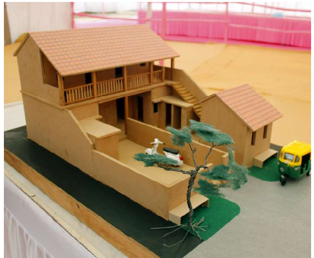
A wooden model of one of the courtyard house designs, with rooms and walls that can be lifted up and taken off, to explain how the house can be expanded in the future.
